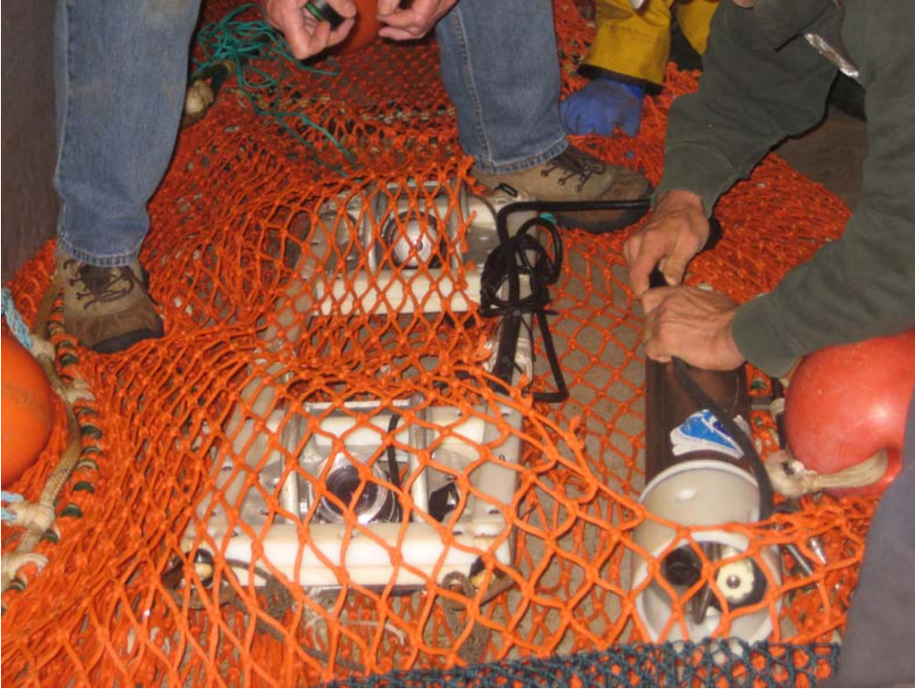
Figure 6. The installation of the video system just aft of the MMED grate in the Nordic 264 trawl.
