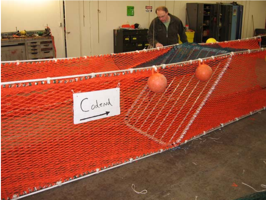
Figure 3. The MMED grate tied into the intermediary panels.
