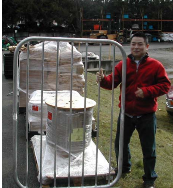
Figure 2. The aluminum MMED grate after construction.
