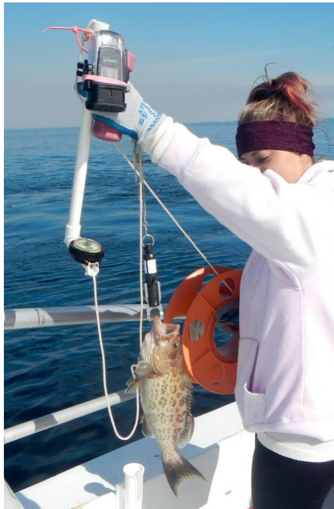
Figure 6. Descender rig with underwater camera. Virb camera in housing with pressure gauge, attached above Seaqualizer device holding fish. Line is spooled on a hand reel for easy deployment and recovery.
