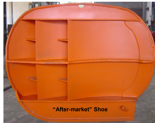
Figure 2. Retrofitted door with an “after market” shoe that increased stability on the sea floor and kept the net in contact with the bottom
