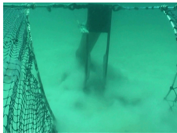
Figure 4. Aft view of the sled with a buoyancy tank being towed between the inside and outside nets
