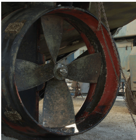
Figure 8. Kaplan propeller seated inside Kort nozzle prior to removal
