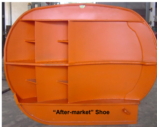
Figure 3. Retrofitted door with an “after market” shoe that increased stability on the sea floor and kept the net in contact with the bottom
