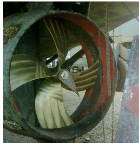
Figure 9. Skewed propeller seated inside Kort nozzle (note wrench on shaft nut)
