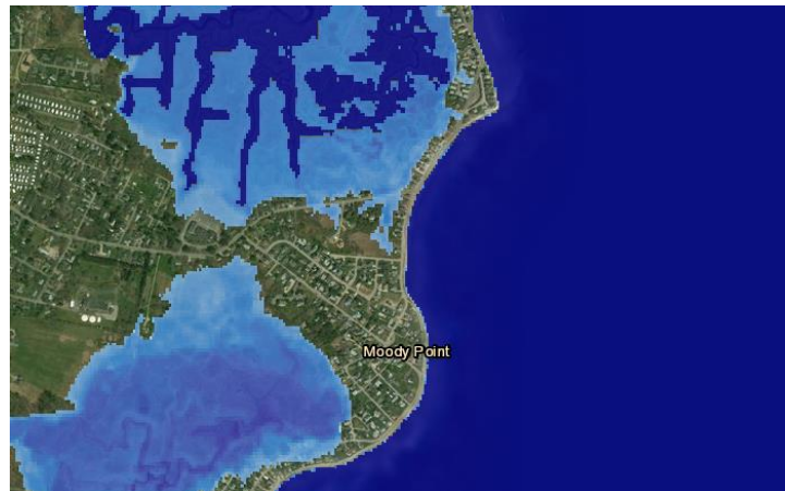
Figure 15: 2 feet Sea Level Rise Effects on Site in Light Blue (DigitalCoast, NOAA)
