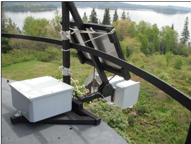
Photo 2-2. Paired acoustic detector deployment. Note: Unit is lashed to tower railing to avoid potential damages in accordance with Maine Historical Preservation Commission recommendations.
