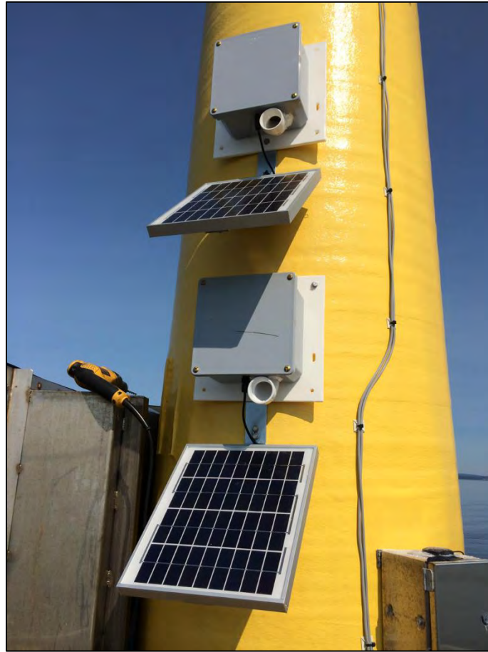
Figure 2-2. Paired acoustic detector deployment, VoltturnUS prototype wind turbine, 2014.
