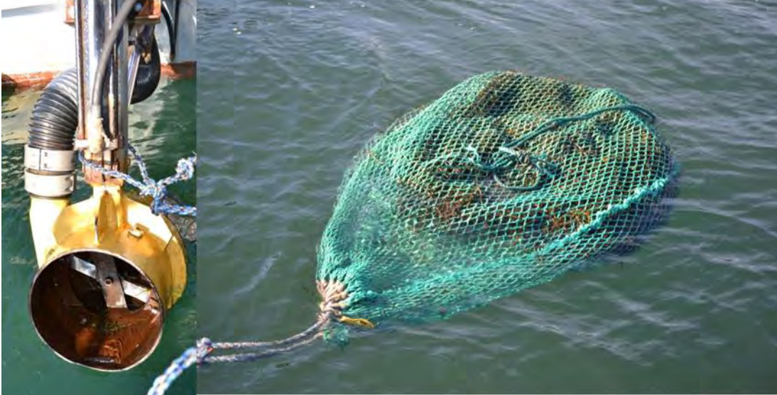
Figure 9. Left. Mechanical harvesting vessel boom cutter. Right. Mesh bag full of mechanically harvested rockweed. Boothbay Harbor, July 2013.
