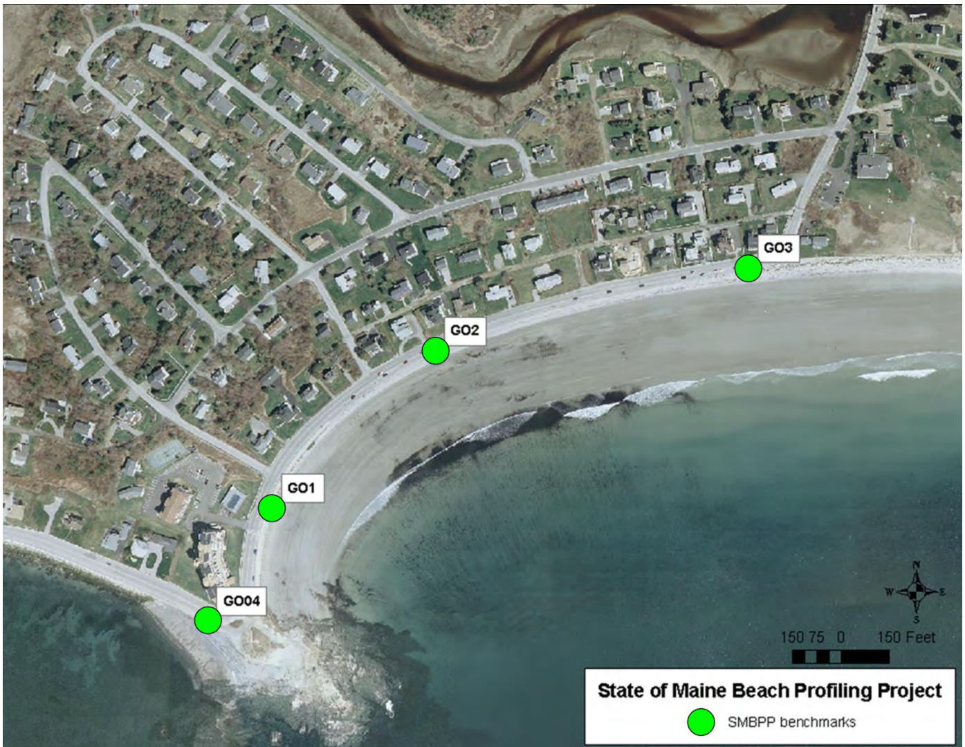
Figure 63. Volunteer beach profile locations at Goochs Beach, Kennebunk. Base imagery from Maine OGIS.
