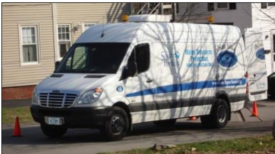
Figure A3. City of South Portland’s closed-circuit television inspection van assessing the condition of the sewer and stormwater systems in the Willard Beach Watershed.
