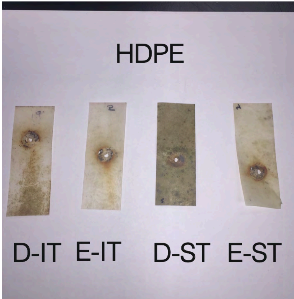
Figure 6. Visual of differences in biomass development at week 4 for HDPE plastic.
