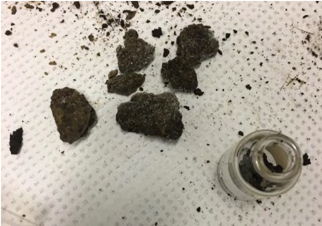
Figure 3. Active layer sediment subsampling, showing ice crystals.
