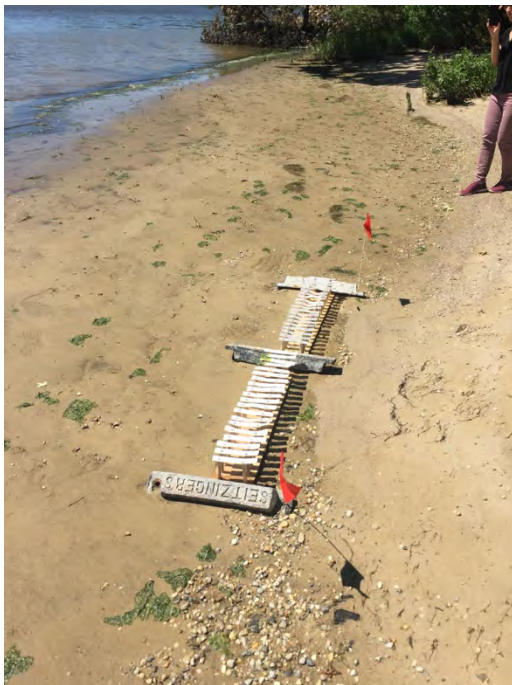
Figure 2. The Intertidal sampling apparatus deployed in the deposition zone.
