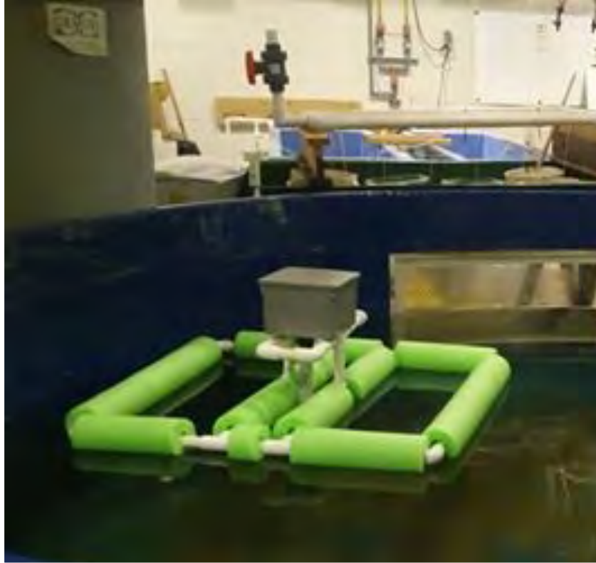
Figure 3. The DACS interior and exterior components fully together. The electrical components sit in the air-tight junction box that sits upon a PVC piping base. That base then sits upon a PVC-noodle base, which allows for it to float. Then stem in a one-inch PVC pipe with holes at the end to assist with water circulation throughout the stem.
