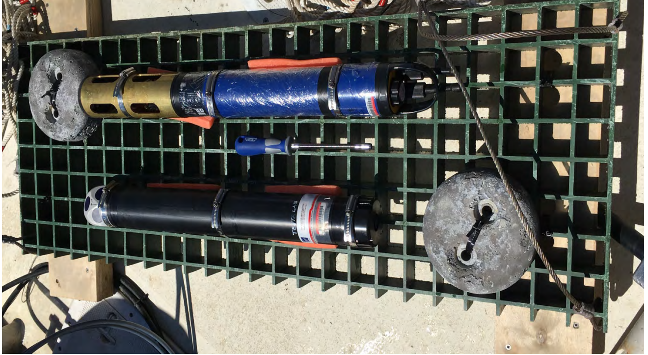
Figure 4: Rigging setup for ADCP and EXO2 sonde deployment. ADCP was set for a deployment while looking up in shallow water, therefore, this platform setup was necessary.
