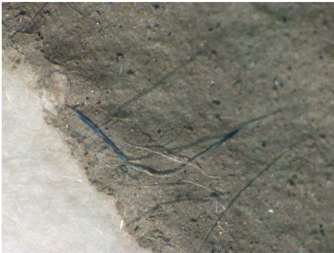
Figure 6. The small filter from the top portion of the SMI unit shows a blue and white pattern synthetic fiber.
