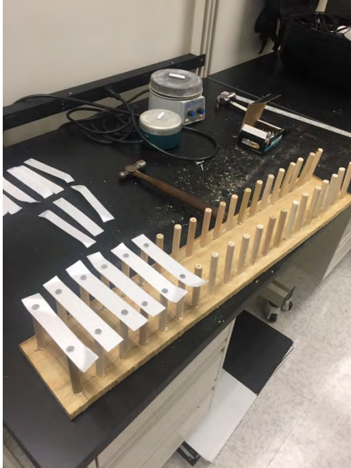
Figure 1. Half built sample board. This picture clearly shows the orientation of the plastic strips and the arrangement of the dowels.
