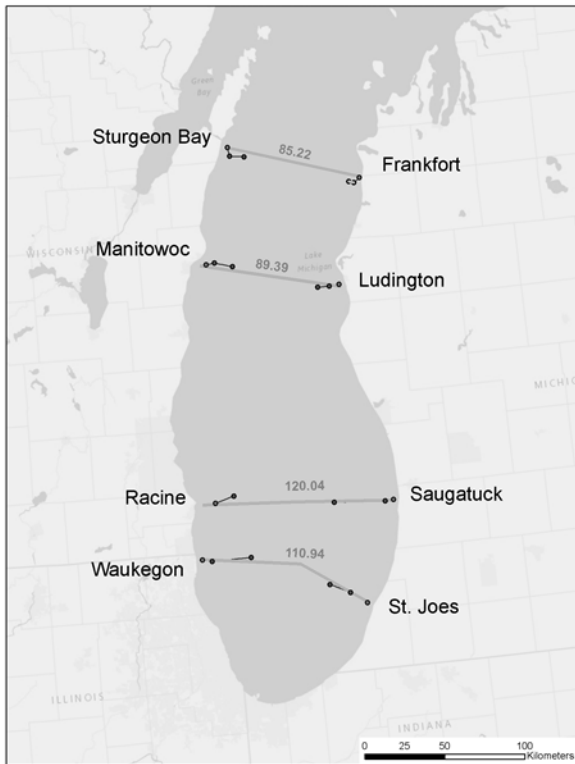
Figure 1. Lake Michigan 2015 CSMI transects with dots indicating vertical CTD casts. Light gray lines represent cross lake transects and distances.
