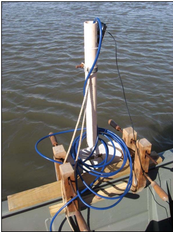
Figure 2. Transponder apparatus and tracking system
