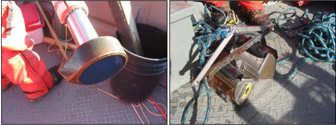
Figure 3. Transponder and benthic grab used to verify sediment characteristics
