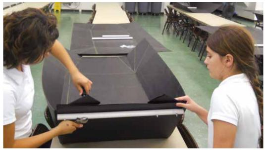
Three layers of plastic are attached to the PVC piece with the fasteners.
