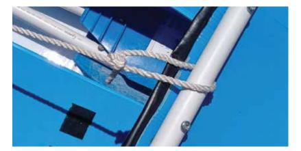
The simplest way is to use about 6' of rope and tie a bowline around the bow.
