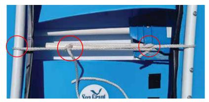
Then loop back under stern piece, go back through the loop at the bow and tie off.
