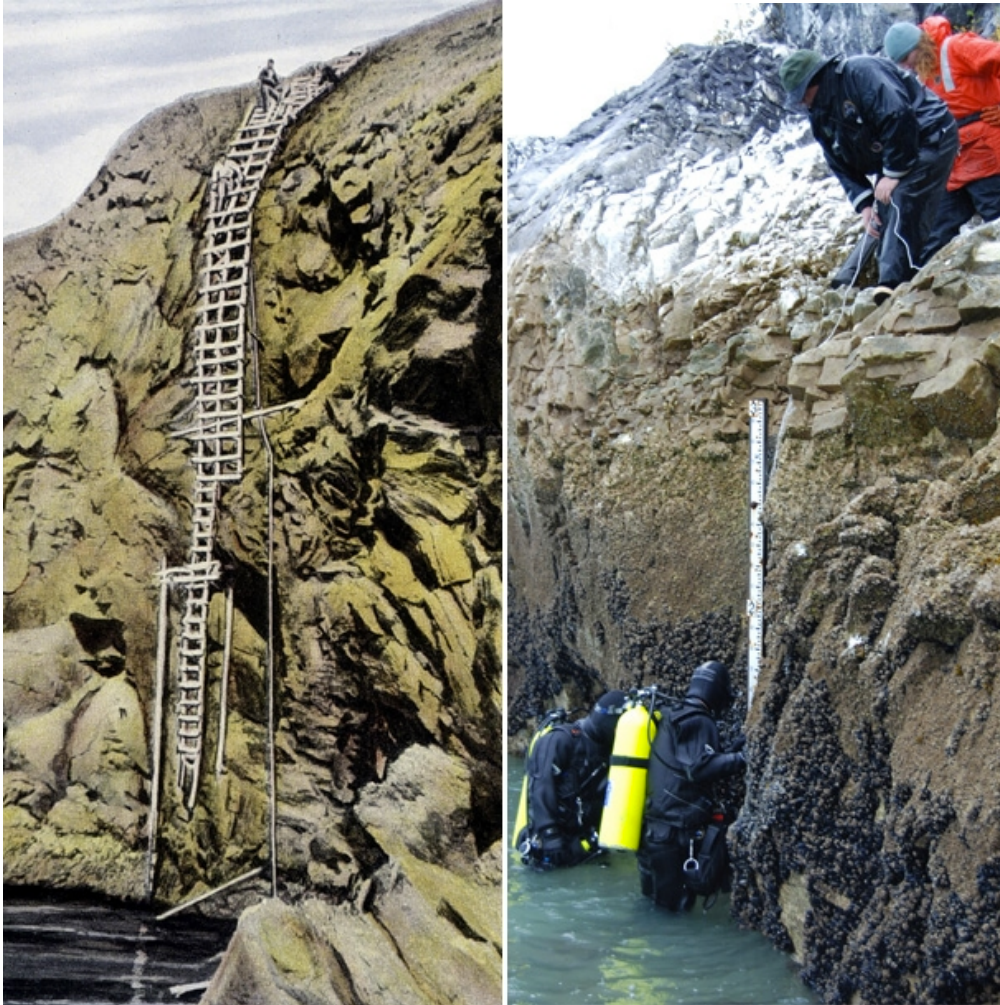
(left) To read the tide gauge at Cape Mordvinof on Unimak Island, Alaska, in 1939, scientists had to descend a 60-foot ladder suspended by wires and stakes. (right) Scuba divers check a cliffside tide staff in Glacier Bay, Alaska in 2010. Historic photo from NOAA Photo Library. Modern photo Ensign Patricia Raymond, NOAA Corps, via the NOAA Photo Library.
