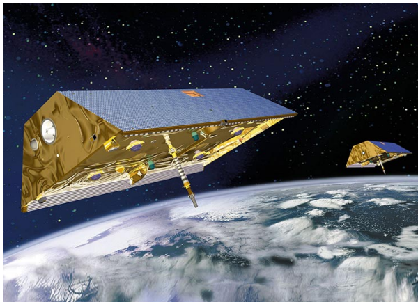
The GRACE twin satellites make detailed measurements of Earth's gravity field. Credit: NASA
