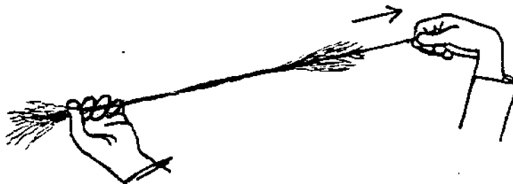
Figure 2. Pulling fibers from a twisted bundle.
