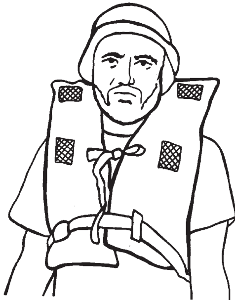
Type II PFD—Nearshore buoyant vest.
