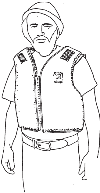
Type III PFD—Flotation Aid—Vest.
