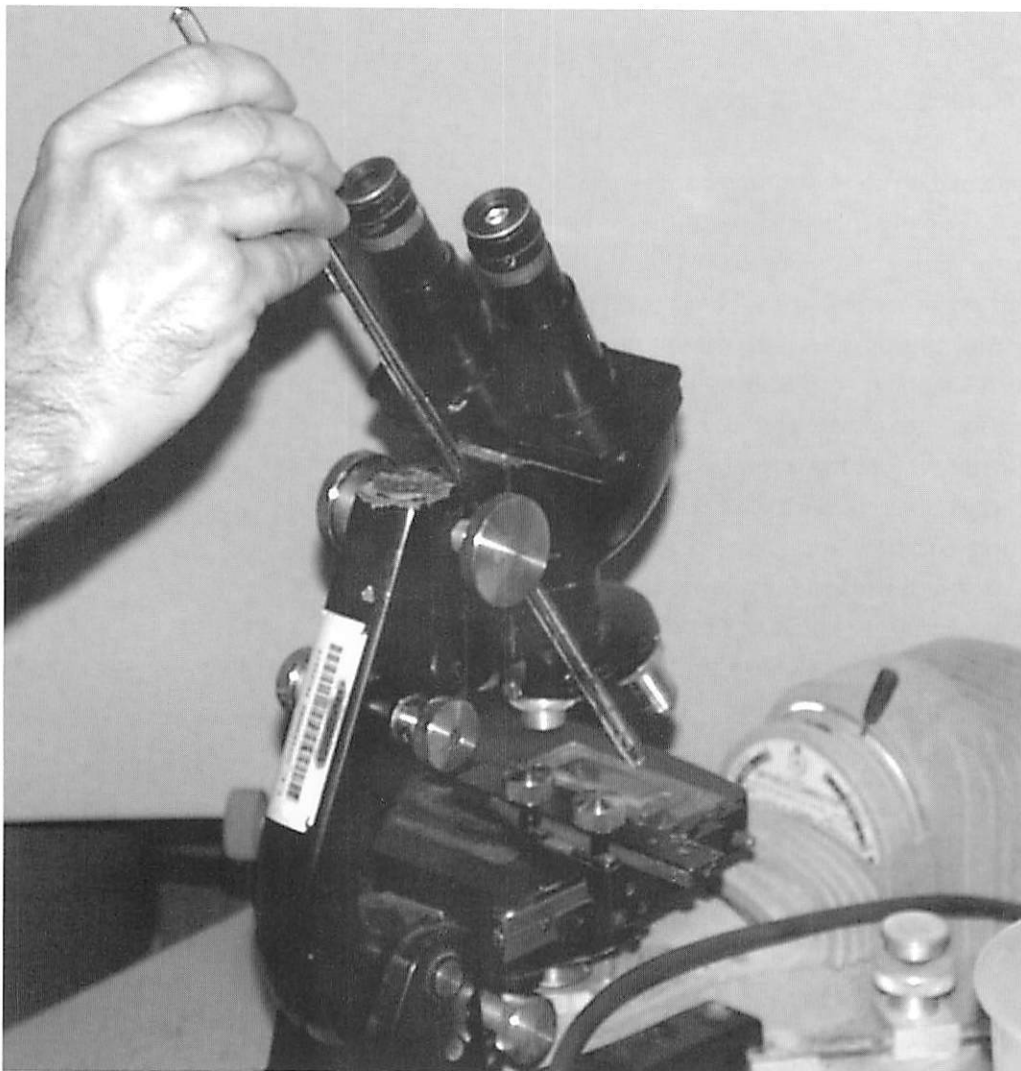
Figure 11. Dispensing a 1-mL sample of egg suspension on a Sedgwick-Rafter counting cell.
