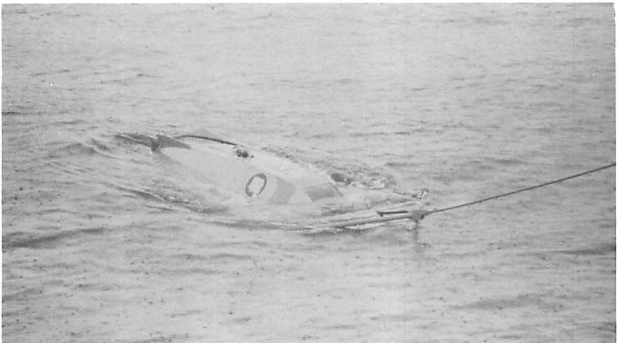
Figure OV-2. RUFAS II breaks the surface after successful tow test in the Gulf of Mexico.
