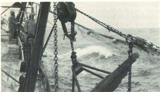
A new semi-automatic trawl door hook-up system being tested aboard the Vincie-N.
