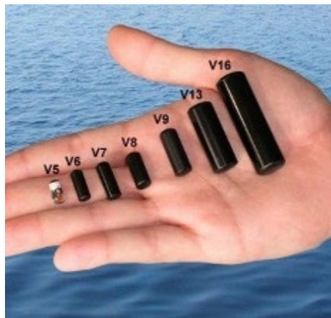
Figure 3. Vemco acoustic tags proposed for use in giant manta rays (V9 and V16).
