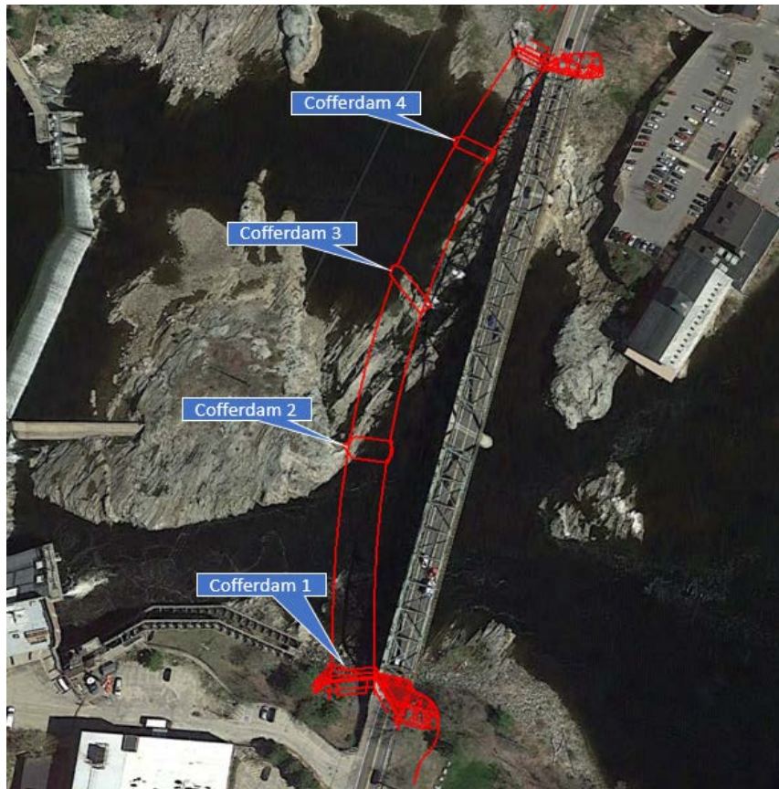
Figure 3: Schematic showing proposed locations of cofferdams required for installation of new Brunswick-Topsham Bridge
