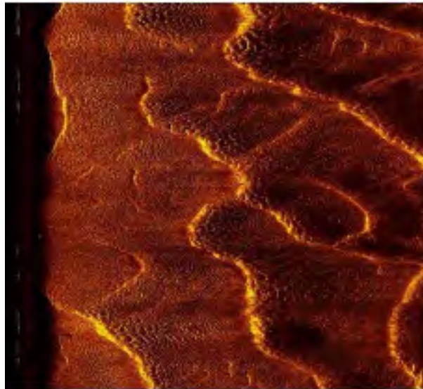
Figure 8 – Sand ripples visible in SSS image (Figure 5 in the BA)
