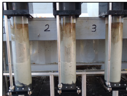
Fig. 2. OSIL multi-corer system (top) and close-up view of sediment core tubes (bottom).
