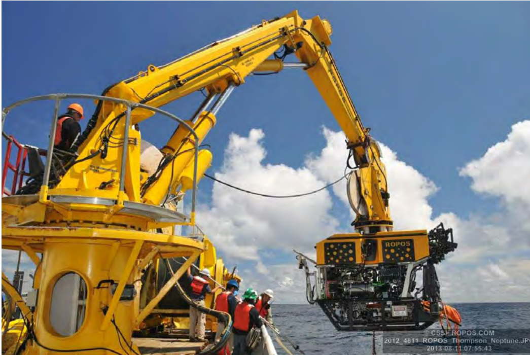
Figure 16. ROPOS with crane-based Launch and Recovery System (LARS) (Canadian Scientific Submersible Facility). ROPOS is equipped with state-of-the-art HD video cameras,
