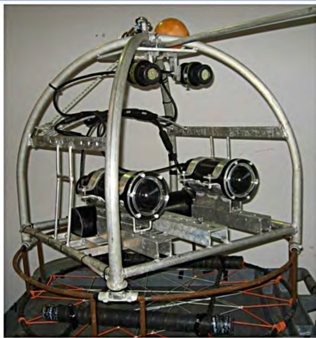
Figure 6. ODFW stereo-video lander system, showing paired stereo-calibrated high-definition Canon Vixia® HFS21 video cameras, and two DSPL Sealite Spheres® (3000 lm, 6000 K) (photo - R. W. Hannah, Oregon Department of Fish and Wildlife).
