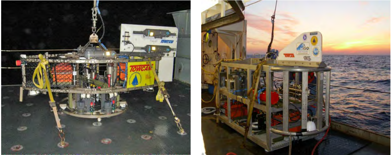
Figure 8. WHOI-MISO TowCam system rigged with water sampling and rock coring capability in 2006 (left) and with DataLink and suction system for Bigelow East Coast Canyons cruise in June 2013 (right)
