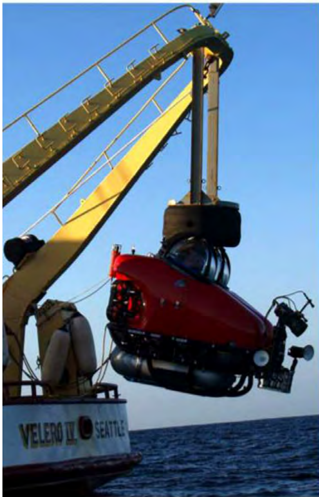
Figure 21. The yellow Delta (right) and red Dual Deepworker (left) research submersibles accommodate one scientific observer and one pilot, and were operated to a maximum depth of 365 m (Delta) and 440 m (Dual Deepworker) at a survey speed of 0.5-1.0 kts.
