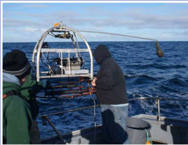
Figure 7. Stereo video lander during deployment – note configuration of bait bag (upper right).
