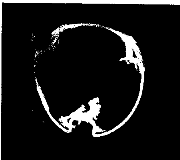
Figure 1d. Radiograph of valve specimen illustrated in Figure 1c. Calcium appears bright white. (Figures 1c and 1d reprinted with permission from Schoen and Hobson 1985).
