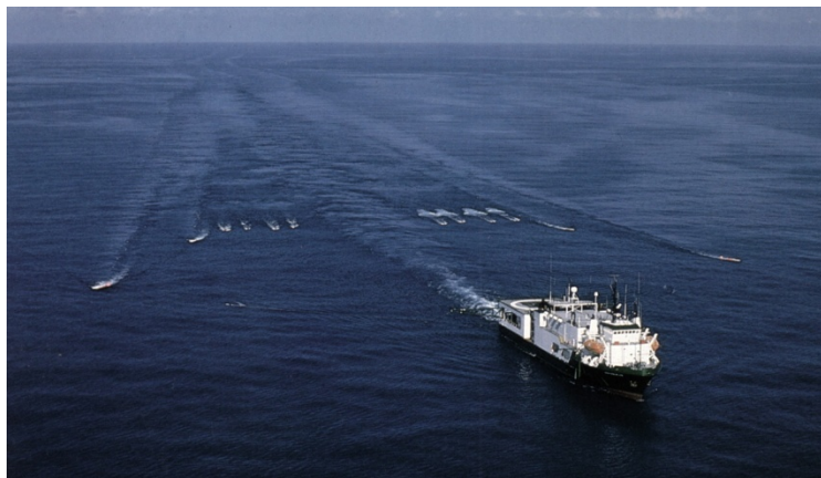
Figure 10: A seismic vessel shooting a 3D marine survey (Credit: Western Geophysical)
