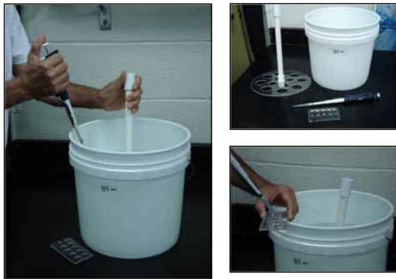
Fig. 8. Sampling ark clam eggs and larvae with a pipette while continuously and evenly suspending them in a bucket using a perforated plunger.
