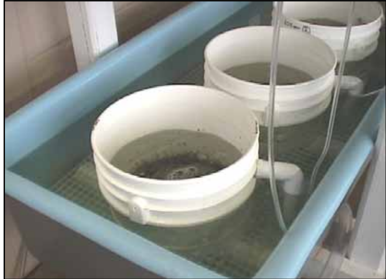
Fig.11. Downwellers in tanks used to rear post-set ark clams.
