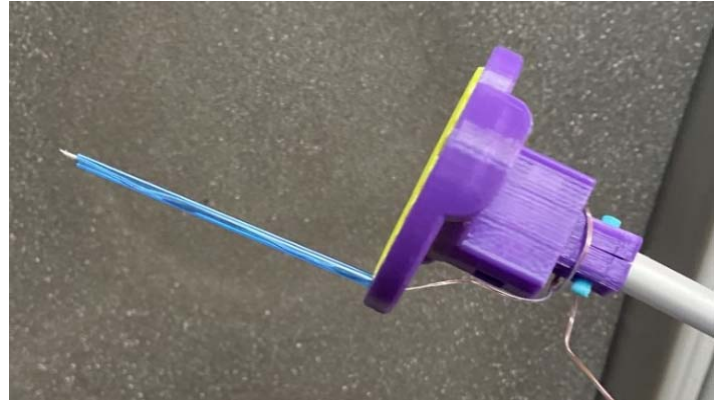
Figure 16: Thermocouple inside of straw cut in half.
