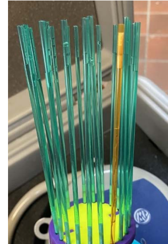
Figure 18: Orange straw showing the thermocouple inserted half-way into the sample.
