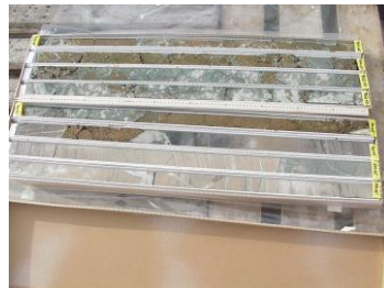
a) Cape Roberts Project drill rig. CRP's mission was to collect samples below the sea floor to document paleoenvironmental changes, the history of the East Antarctic ice sheet, and the tectonic history of the Transantarctic Mountains (Photo credit: John Wrenn). B) Sediment core samples recovered during the 2001 CRP campaign near McMurdo station (Photo credit: Sophie Warny). C) Palynologist analyzing microscopic samples of fossilized Nothofagus pollen (displayed on screen). Samples were recovered from cored sediments buried below Ross Sea (Photo credit: Sophie Warny).
