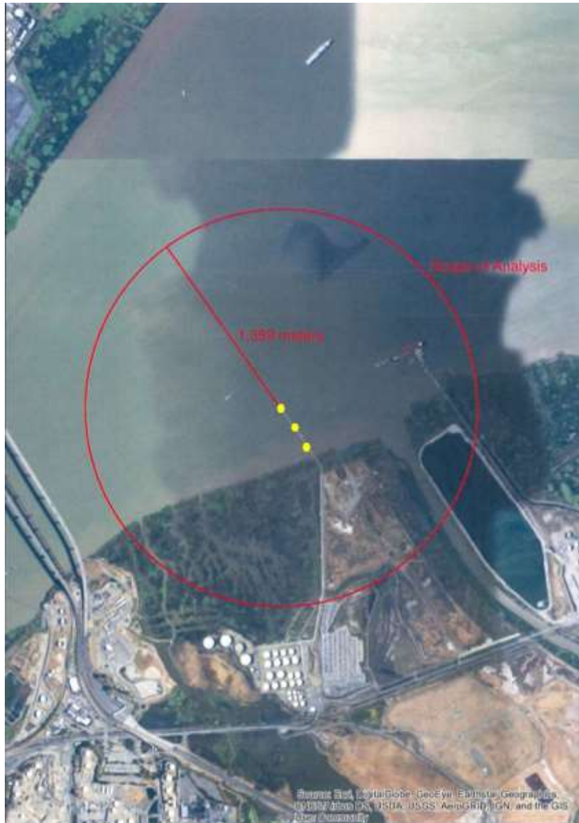
Figure 1. Action Area for the Martinez Marine Terminal Repair and Retrofit Project. Yellow dots represent the general locations of piles to be installed. The open water area inside the red line illustrate the extent within which behavioral effects may occur to fish resulting from impact hammer pile driving.
