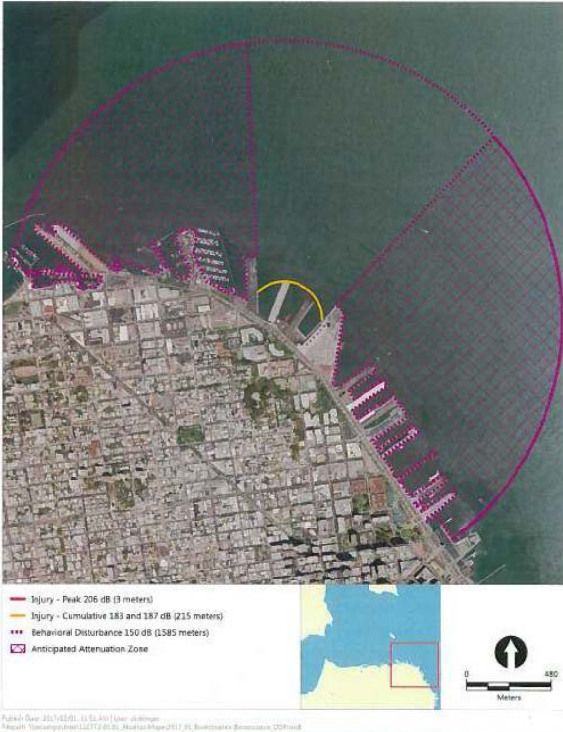
Figure 3. Action Area extent at the Pier 31.5 Project site (~ approximately 405 acres) is the open water arc inside the purple lines (non-hatched area) within which behavioral effects may occur to fish resulting from pile driving sounds. The area within the yellow circle (~approximately 32 acres) is the zone of potential barotrauma injuries to fish resulting from cumulative sound exposure levels (cSEL) generated by pile driving over a full day.
