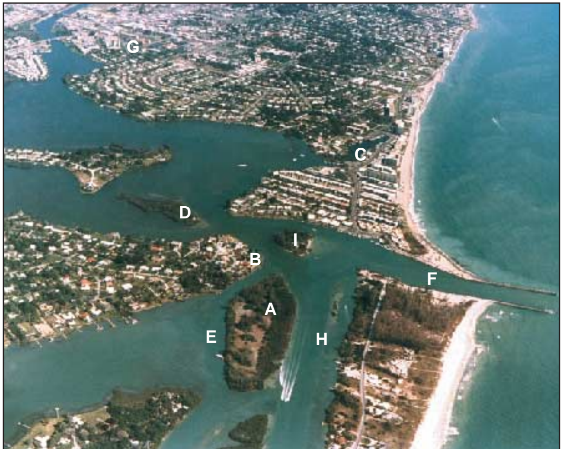
Photo 5. Aerial view south of Venice Inlet, around 1990, showing new and original (relict) ICW channel
