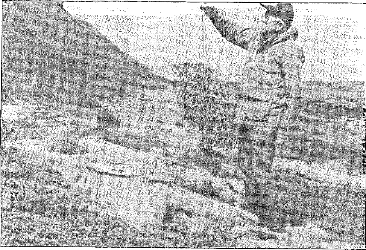
Figure A-3.--Weighing trawl-web fragment with Pesola spring scale.
