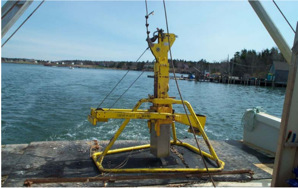
Figure 7. Ocean Instruments box corer used during survey.
