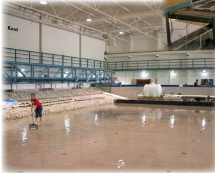
Scott Socolofsky and Kuang-An Chang of Texas A&M University are using the Coastal Engineering Laboratory's shallow wave basin to further understanding about the mechanisms of water exchange through inlets between the open Gulf and bays and their impact on the water quality of Texas' estuaries.
