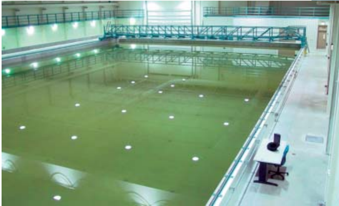
The shallow wave basin of the Reta and Bill Haynes '46 Coastal Engineering Laboratory at Texas A&M University is being used in research studying exchange processes between estuaries and the open Gulf.
