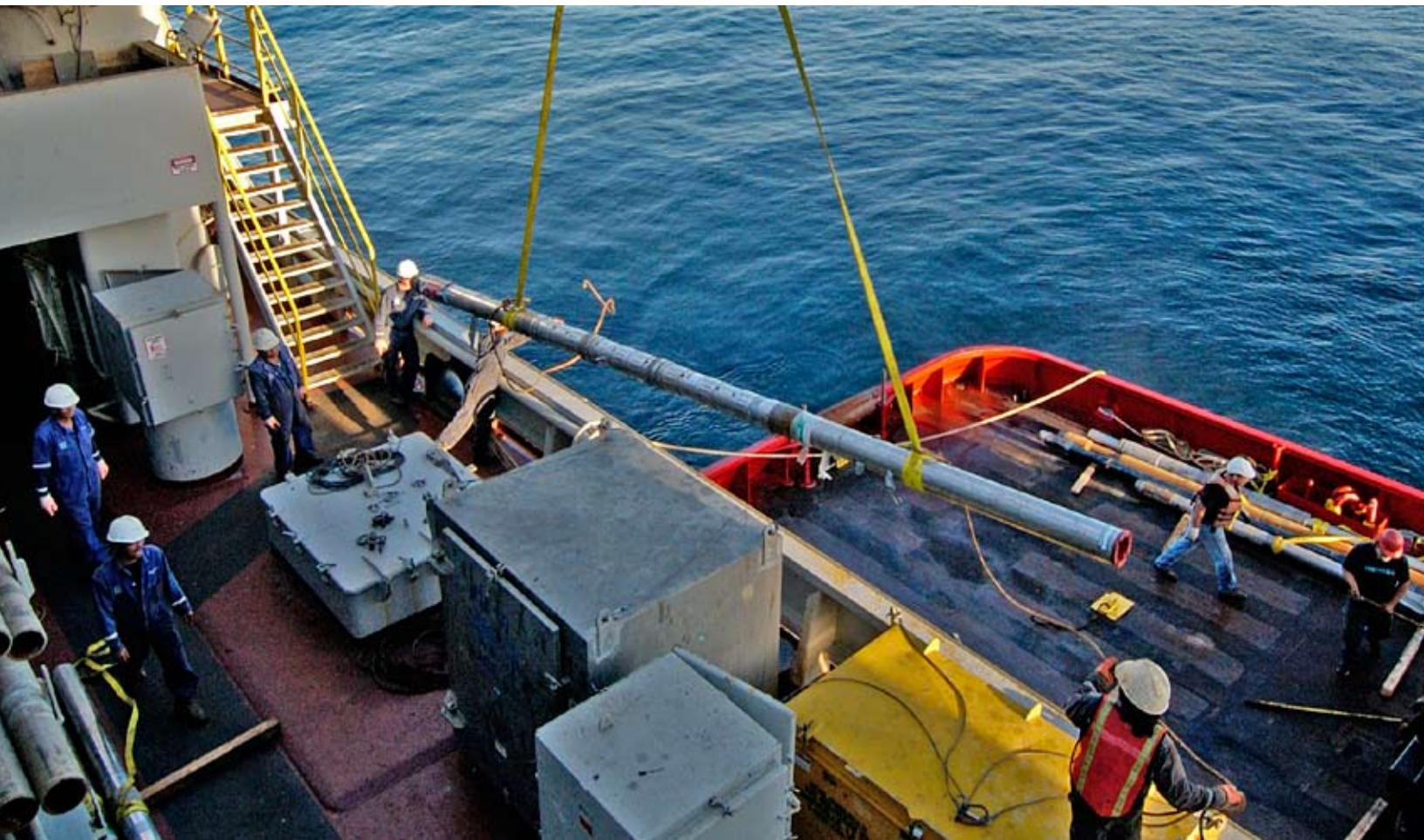
Crew members load drill pipe aboard the scientific drilling vessel Joides Resolution .
