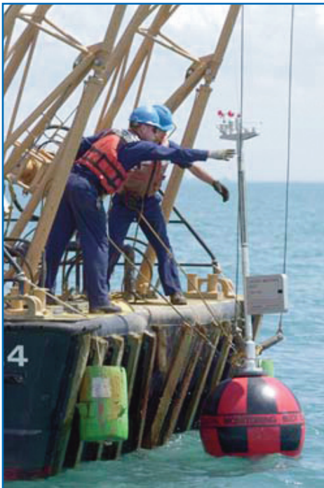
Researchers deploy an automated meteorological buoy in Lake St. Clair, one of the components of an environmental monitoring network developed by UM researcher Guy Meadows.
