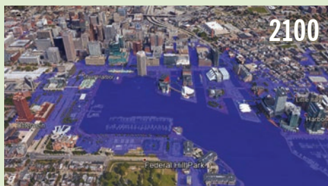
MODELED INUNDATION of downtown Baltimore during Hurricane Isabel in 2003 (top) projected to 2100 (bottom) under the IPCC RCP 8.0 climate scenario. GRAPHIC COURTESY OF MING LI, GERONIMO.HPL.UMCES.EDU/MINGLI
