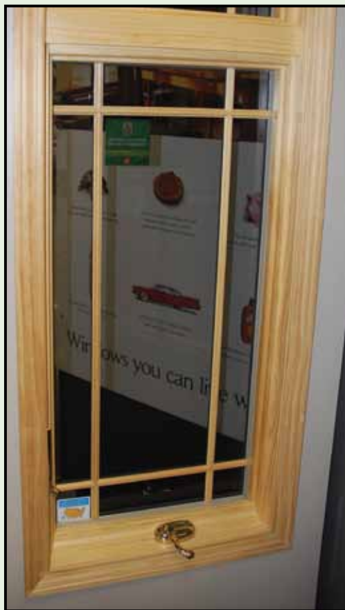
Figure 26. This attractive window can be fitted with energy-efficient glass, impact-resistant glass, or both. The impact-resistant glass consists of a laminate or film sandwiched between two glass panes. The frames are reinforced and the hinges have an extra fastener to withstand high winds. During a wind event, debris may crack the glass, but the laminate will hold the windowpane together in the frame and prevent breaching of the wind- and rain-resistant envelope. After the storm, the glass will need to be replaced.
