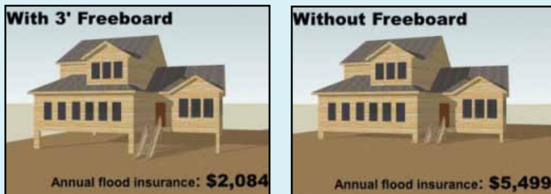
Figure 4. Adding a small amount of height has very little effect on the look of a home. Source: Texas Storm Smart Coasts.
