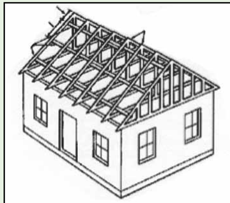
Figure 8. Trusses are built with a peak at the ridgeline of the roof, which forms an A-shaped pattern known as a gable end. During a hurricane, the gable end is subject to high wind intensities that may damage other trusses if not properly stabilized. Source: FEMA’s “Against the Wind” brochure (FEMA 247).
