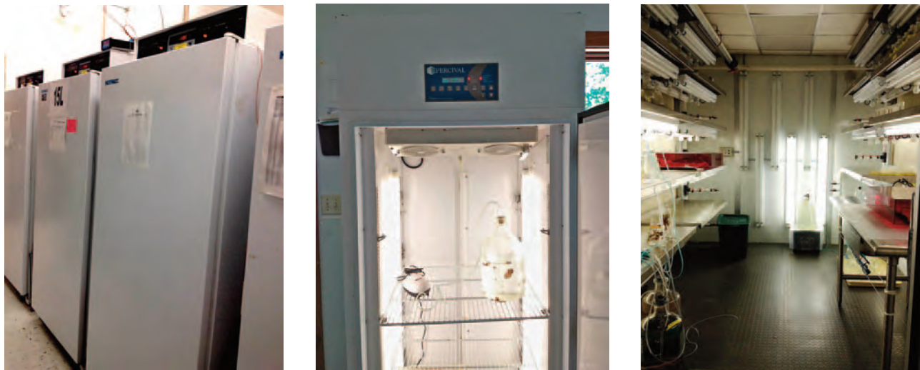
Figure 2.5. Environmental culture chambers, also known as incubators. These can be any size, and can be purchased commercially or can be homemade. Environmental chambers all have a means of temperature control, a light source with photoperiodic control, and aeration. Left: Hotpack brand incubator. Middle: Percival Biological incubator, Right: Room-sized environmental chamber.
