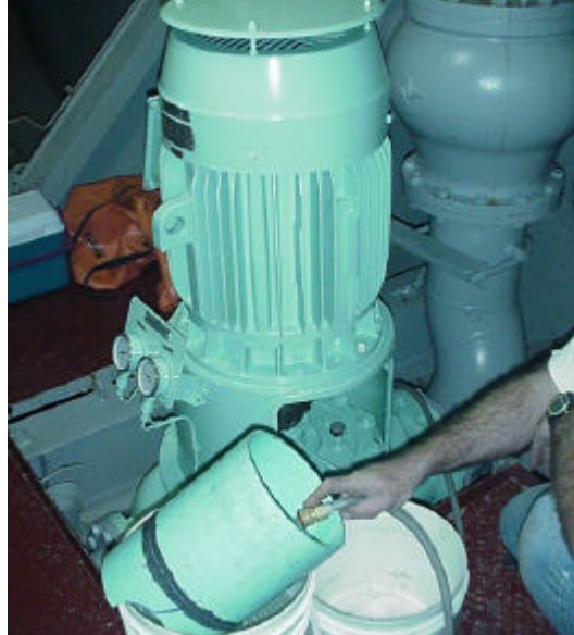
Figure 3. Example of a ballast water pump in the engine room where the ballast water samples were collected. Note the 20-um mesh screen used to collect the phytoplankton and zooplankton specimens.
