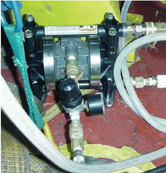
Figure 2. The lightweight air-pump (left) used to obtain samples of ballast water through the sounding pipes (right). The air-pump was connected to a scuba diving tank by means of quick disconnect fittings.
