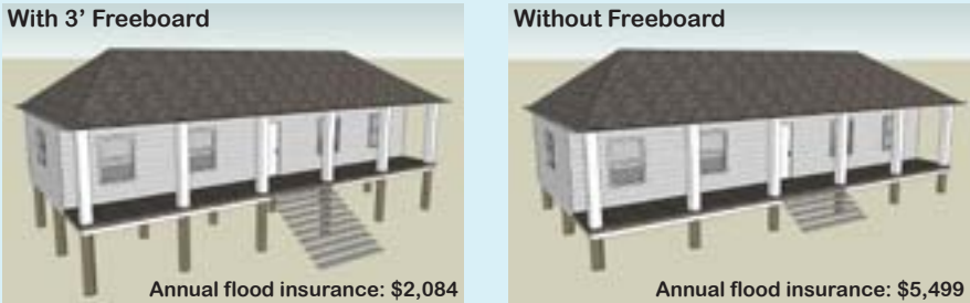
Figure 2-6. In this example, adding a small amount of height has very little effect on the look of a home, but resulted in a substantial flood insurance savings. 8 Source: StormSmart Coasts-Alabama
