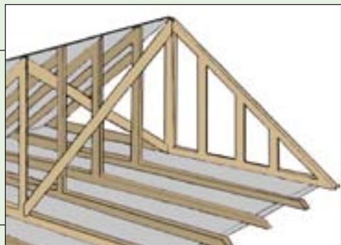
Figure 4-4. Diagonal braces form an X pattern from the top center of the gable end to the bottom center of the fourth truss and from the bottom center of the gable end to the top center of the fourth truss. The same screws as for lateral bracing are used. Source: FEMA's "Against the Wind" brochure 247
