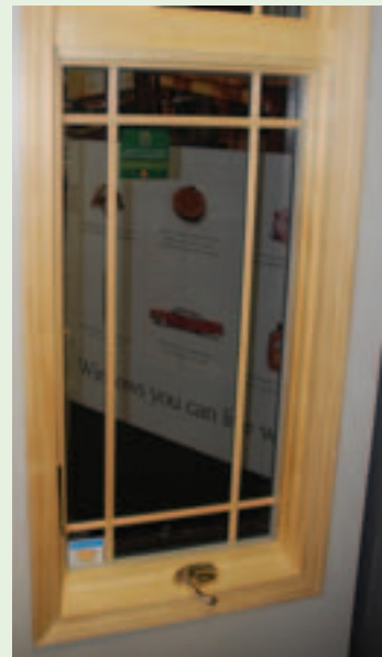
Figure 4-20. This attractive window can be fitted with energy-efficient glass, impact-resistant glass, or both. The impact-resistant glass consists of a laminate or film sandwiched between two glass panes. The frames are reinforced and the hinges have extra fasteners to withstand high wind events. During a wind event, debris may crack the glass, but the laminate will hold the window pane together in the frame and prevent breaching of the wind- and rain-resistant envelope. After the storm, the glass will need to be replaced.
