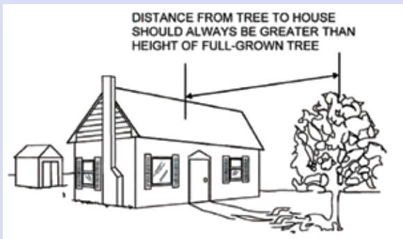
Figure 4-49. FEMA recommends keeping trees a distance greater than the height of a full grown tree. This will prevent roof damage from strong winds and also reduce risk that leaves will fall on your roof and enter the water catchment system.
