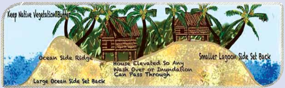
Figure 4-55. From the UH Sea Grant publication “A Landowners Guide to Coastal Protection.” The ocean side of the atoll receives more wave energy and consists of coarser grained and steeper ridges or berms. The lagoon side has smaller ridges and finer sediment. It is important to build and maintain migratory and fixed ridges or berms. Also re-vegetate the shoreline below the high water mark with mangroves and above with other suitable salt-resistant varieties.
