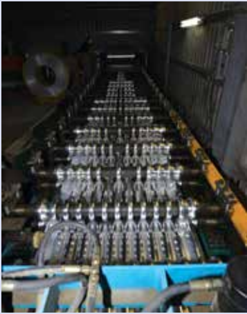
Figure 4-51. An aluminum press and cutting sheet in Majuro can make metal corrugated roof and gutters of different dimensions. This can help to ensure proper overlap of aluminum roofing sheets (two ridges of overlap – see Figure 4-23). In addition, aluminum gutters can be created that are 4, 5, or 6 inches in width. The larger gutter width will maximize water capture during a rain event.
