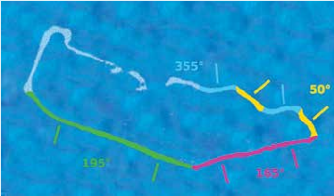
Figure 2-20. Majuro has been color coded into four shoreline sectors, depending on the orientation of the coastline with incoming waves. The shoreline sectors are perpendicular to waves coming in at 50, 165, 195, and 355 degrees of the compass. Each color represents a forecast of potential inundation. No forecasts are explicitly provided for the gray-shaded land areas.
