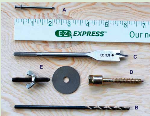
Figure 4-31. Many panels have permanent fastenings attached to the house. (i) After attaching the panel to the frame with two duplex nails (A), (ii) holes are drilled with the bit (B) into the panel and wood frame, (iii) then a spade wood boring bit (C) cuts wider holes into the panel and frame, (iv) and a lag screw anchor with female receptor (D) is screwed into the wood frame, (v) and the panel is attached with washer and wing nut (E).
