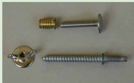
Figure 4-32. Another method of attachment uses brass grommets (upper left) that are screwed into the wood frame. A wide head screw attaches the panels. Lower screw and washer wing nut are used to hold the two top corners. This is the method used in Figure 4-20.
