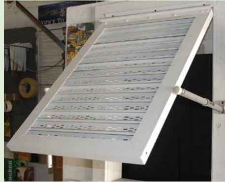
Figure 4-10. As a storm approaches, the Bahama shutter is pushed down against the wall and anchored with stainless steel bolts through the frame into anchor sleeves in the wall. Photo courtesy of Hurricane Secure.
