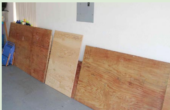
Figure 4-28. Once the panels are created, they can be stored in the garage and take up minimal space if stacked neatly along the side of the garage, with the smallest pieces closest to the wall. Panels should be checked each year for any warping or rotting and replaced as needed.
