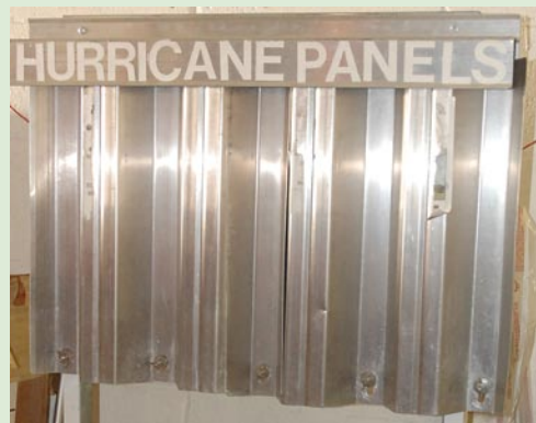
Figure 4-13. Although installation varies, this example shows panels that slip into a track above the window. The bottoms of the panels are secured by bolts that are permanently attached to the window. Photo courtesy of Hurricane Secure.
