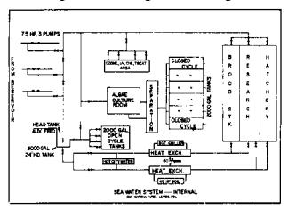
Internally, a dual-pump, head-tank system delivers and distributes up to 400 gpm of a combination of heated, cooled, and ambient temperature seawater.
