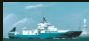
The 274-foot research vessel Atlantis is the platform from which Alvin operates. Atlantis can carry up to 60 people, including crew, scientists, and technicians. The ship features hangars for Alvin and ROVs (remotely operated vehicles), portable labs, a machine shop, library, laundry, and inflatable rescue boats.
