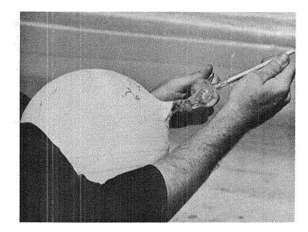
FIGURE 2 - Purging procedure shown using 5-liter flask.
