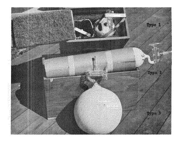
FIGURE 1 - Three types of sampling flasks currently in use.
